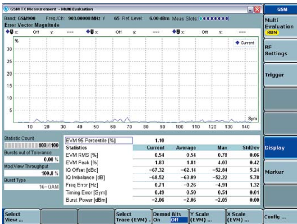
Modulation analysis screen: EDGE Evolution TX measurement.
